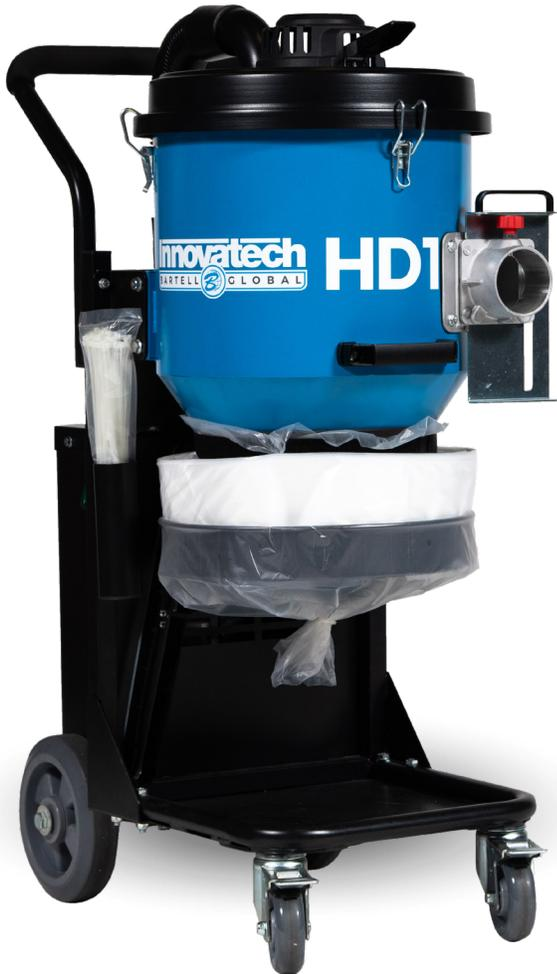
**TWO-STAGE HEPA FILTER SYSTEM WITH JET-PULSE FILTER CLEANING**
