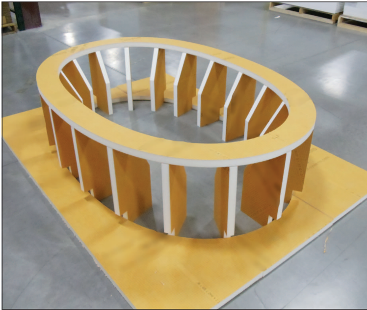
Building panels for tub surrounds were cut at the factory and sent in kit form for assembly at the resort in Grand Cayman Islands.
