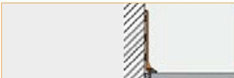
**16.2 Schluter®-DESIGNBASE-SL** is a finishing profile used as an alternative to baseboards. The profile is available in anodized aluminum, color coated aluminum and stainless steel. It features a clean, finished look and is simply attached to the wall with a suitable adhesive. The profile can be equipped with an optional sealing lip to help protect
