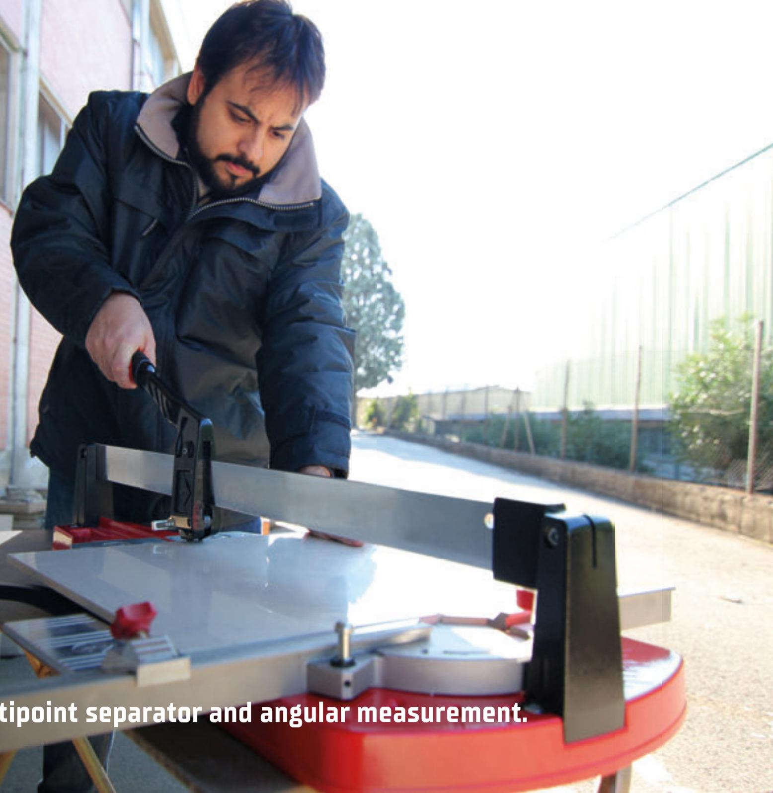
**Single guide with multipoint separator and angular measurement.**
