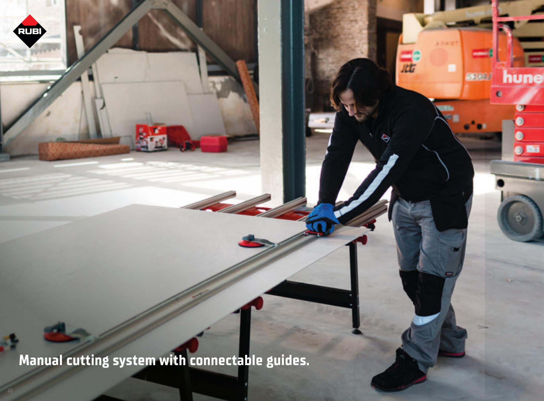
**Manual cutting system with connectable guides.**
