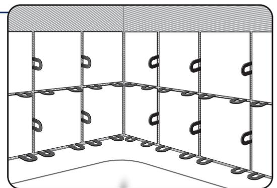
QEP® Horseshoe Shim Tile Spacers are ideal for spacing and aligning marble, granite, stone, and large format tile installations. They are engineered to produce a grout joint, and to quickly and easily space, and align horizontal and vertical tile. They are injection molded for dimensional accuracy and do not compress under heavy loads, making them especially helpful in vertical installations. QEP Horseshoe Shims are easy to clean, reusable, and packaged in a convenient recyclable pail.
