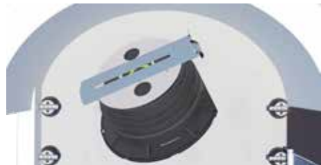
7. Place the SUPACLPP perpendicular to the wall.
