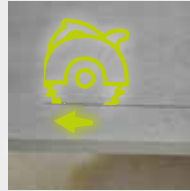
D4. Cut the tile. The dimension of the tile is equal to the distance between the BSJ profile and the SUPACLPB base clip.
