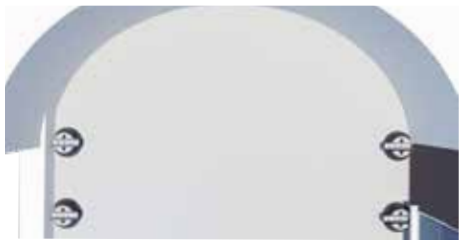
4. Place the pedestals in the positions indicated on the layout diagram.
