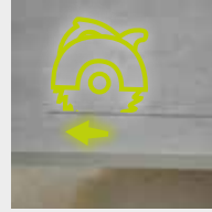
D4. Cut the tile. The dimension of the tile is equal to the distance between the SUPACLPT clip and the SUPACLPB clip.
