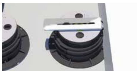
16. Position the SUPACLPP spacer clip.
