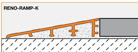
**1.8 Schluter®-RENO-RAMP** is designed to provide a smooth transition between tile coverings and floor coverings at lower elevations or finished concrete, particularly in commercial applications where wheel carts are used (e.g., bakeries, hospitals, etc.). The profile is available in anodized aluminum. RENO-RAMP features a trapezoid-perforated
