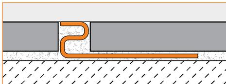
**1.6 Schluter®-DECO** is designed to provide decorative lines within tile coverings and edge protection at transitions from tile coverings to other same-height surface coverings, such as wood or carpet. The profile is available in stainless steel, solid brass, chrome-plated
