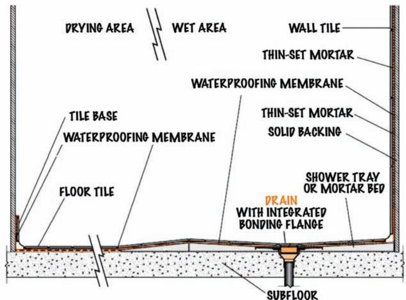
When recessing the floor is not an option, a ramp may be provided in lieu of a curb. The wet area is sloped to the drain to contain water during shower use.
