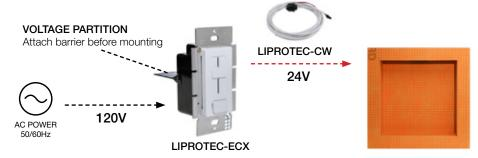
Note: Main power (120V source power) must come through the bottom of the switch box.
