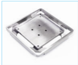
02 Premium tileable drain cover for Fundo Primo and Ligno: can be tiled with epoxy glue/adhesive or wedi Joint Sealant- used with 1/4 inch (6.4 mm) high tile or stone.
