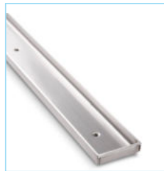
13 Exclusive tileable drain cover for Fundo Riolito: can be tiled with epoxy glue/adhesive or wedi Joint Sealant- used with 1/4 inch (6.4 mm) and 1/2 in. (12.7 mm) tile/stone (reverse cover). Drain cover can be adjusted from +3/16 in. to +1 in. from the Riolito base surface (depth for tiling 11 mm).
