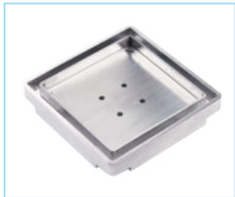
03 Premium tileable drain cover for Fundo Primo and Ligno: can be tiled with epoxy glue/adhesive or wedi Joint Sealant- used with 3/8 inch (9.5 mm) high tile or stone.
