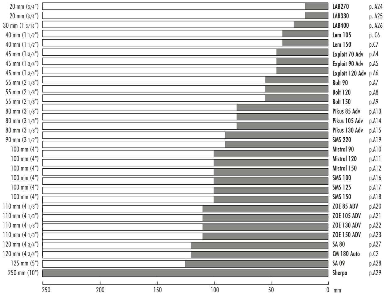
MAX THICKNESS OF CUT (DOUBLE PASS)
