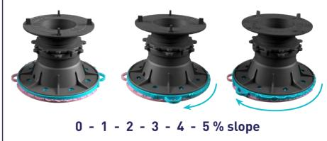
When several pieces are combined we can get all the inclination percentages lower than the maximum slope. We use several regulators to find the exact inclination. Each tab that we rotate to the regulator we add 0,25° of inclination
