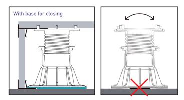
The bottom sheet fits perfectly to the base for vertical closing. In this way, the entire base of the Pedestal is supported correctly and has no reduction in resistance.
