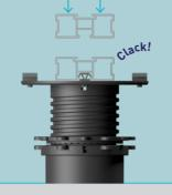
Simply press the joist on the clip and it will be safely anchored to it.
