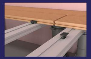
4º Fix the slats to the joist by means of
