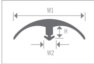
Regular T Cap for use where adjacent floors meet and color coordination is important. For residential or light traffic area. Made for height differentials up to 5/8". Fits wide channels such as CM1655, CM1755, CM1759, CM1140, CM14270, CM14271.
