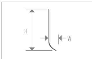
Protects bath tub and flooring from scratches and water damage. Applied where flooring meets base of tub.
