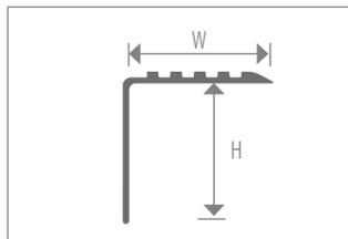
Drop Overlap Nosing. Used over LVT or resilient flooring. Protects edge of floor covering from damage at step face and provides extra traction for safety.
