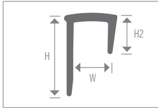
Square Cove Cap for use when coving carpet up to 5/16" thick and where a square look is required. Available with peel and stick tape or dry back.
