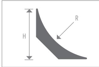
Rigid Cove Former. Used with carpet or resilient flooring to support cove area of flooring material. Score and snap to size for easy installation.
