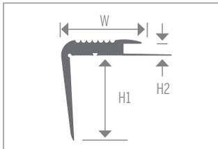
Designed for insert-style installations of carpet or carpet tiles when installed on steps. The flexible lip covers the cut edge of the carpet. Features a patent pending "glue lock" dovetail design on underside of the top face and a relief notch in the nose. These new features both secure and simplify installation.
