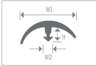
Regular E Cap for use where adjacent floors meet and color coordination is important. For residential or light traffic area. Made for height differentials up to 3/8". Fits wide channels such as CM1655, CM1755, CM1759, CM1140, CM14270, CM14271.
