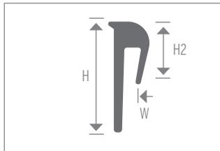
1/8" resilient cove cap for use when coving resilient floor up to 3/16" thick. Peel and stick tape for easy application.
