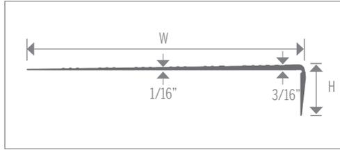
Standard duty Stair Tread to suit most commercial applications. Safety grip top rib pattern.
