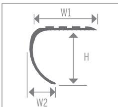
Bull Nose designed to be used with round nosed stairs. Flexible round nose allows for easy installation. 5/8" return helps to hide underside of stair.
