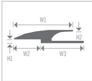
Carpet to Tile Reducer. Creates an attractive, safe transition between carpet and 1/8" flooring. The edges of both floor coverings can easily be tucked in to protect them from damage. The bottom lip is designed to enable the carpet and molding to be glued together and secured to the floor.
