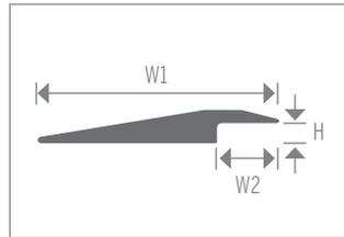
Overlap Tile Reducer for use with resilient or LVT flooring from 0.080 - 0.125" thick.
