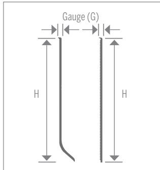
High quality rubber Cove Base manufactured using 100% virgin materials. Advanced co-extrusion technology allows for a tough scuff-resistant surface while maintaining overall flexibility and ease of installation.
