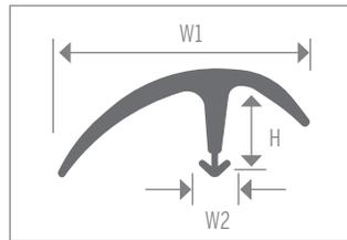
Regular E Cap for use where adjacent floors meet and color coordination is important. For residential or light traffic area. Made for height differences up to 5/8". Fits wide channels such as CM1655, CM1755, CM1759, CM1140, CM14270, CM14271.
