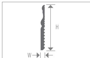
**Estate Base** made of heavy gauge vinyl. Smooth satin finish and intrinsic flexibility helps hide substrate irregularities. Deep grooves and several uniquely - shaped surfaces simulate milled wood moldings. Easy to cut and install.
