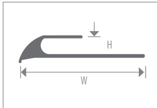
Insert Reducer for glue down carpet installations. Lip flexible up to 5/16". Also available with Peel & Stick back.
