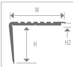
Designed as an "Over the Top" style installation of VCT, LVT and LVP type floors when installed on steps. Features a patent pending "glue lock" dovetail design on underside of the top face and a relief notch in the nose. These new features both secure and simplify installation.
