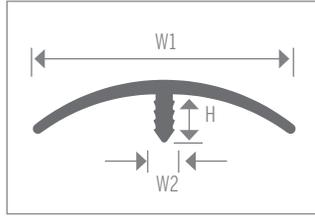
Commercial T Cap for use where adjacent floors meet and color coordination is important. E- Cap for use on height differentials under 5/8". Made for high traffic commercial purposes. Use with CM1651, CM1659, CM1751, CM1752.
