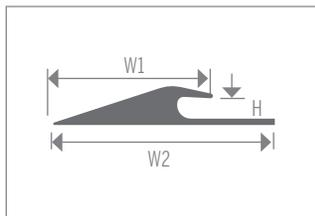
Insert Reducer for glue down carpet installations. Lip flexible up to 3/8". For light commercial or residential use.
