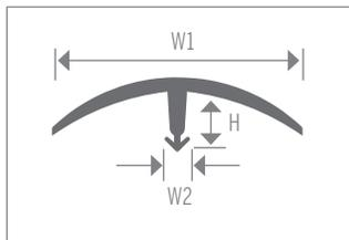
Regular T Cap for use where adjacent floors meet and color coordination is important. For residential or light traffic area. Made for height differentials up to 3/8". Fits wide channels such as CM1655, CM1755, CM1759, CM1140, CM14270, CM14271.
