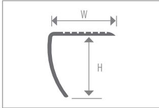
Overlap Nosing. This Rubber/Vinyl composite nosing has large legs to help cover damaged area or stairs with unusually large drops.
