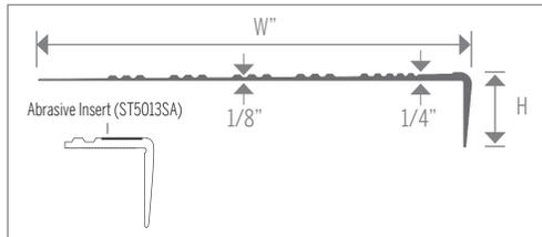
Heavy Duty Commercial Stair Tread. Safety grip top rib pattern. Easy flex leg for set back risers.
