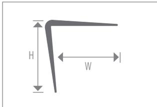
Flexible Vinyl Corner Guard: Corner protector for walls and doorways where a bumper guard is needed. This product will not shrink, crack or chip like rigid plastics.
