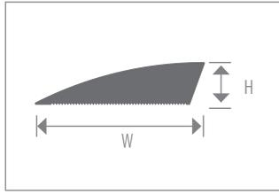
The butt-type reducer is designed for applications where you need to reduce down from a 3/8" height differential and require a smooth sloping transition to the adjacent flooring surface.
