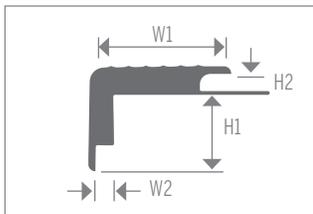
Commercial friction-double insert nosing. For carpet or tile up to 3/8" thick. Notched for easy installation.
