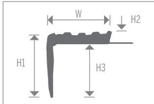
Commercial Nosing. Designed to butt to 3/8" ceramic tile, providing excellent traction.
