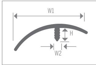
Commercial E Cap for use where adjacent floors meet and color coordination is important. E- Cap for use on height differentials under 5/8". Made for high traffic commercial purposes. Use with CM1651, CM1659, CM1751, CM1752.
