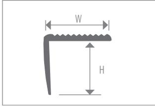
Square Nose covers and protects leading edge of stairs. Use over vinyl and sheet goods. Excellent slip resistance. Smaller profile nosing provides a clean finished edge.
