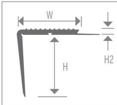
Designed for Butt-style installations of various flooring types like VCT, LVT and some low pile carpets when installed on steps. Features a patent pending "glue lock" dovetail design on underside of the top face and a relief notch in the nose. These new features both secure and simplify installation.
