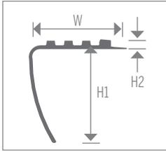
Drop Butt - Type Nosing. Use to butt up to 1/8" LVT tile or resilient floor. Protects edge of floor covering from damage at step face and provides extra traction for safety.
