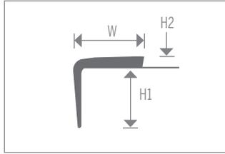
Commercial Single Butt-Type Nosing. For butting up to 1/4" tile or carpet.
