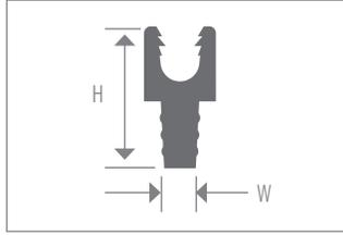
Channel Extender. Made of Rigid PVC. Can be used on ceramic tile installations when inserted into track. This extender increases effective height of channel by 3/8".
