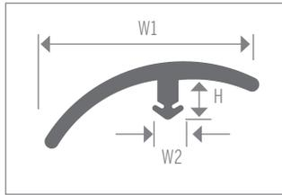
Regular E Cap for use where adjacent floors meet and color coordination is important. For residential or light traffic area. Made for height differentials up to 5/8". Fits wide channels such as CM1655, CM1755, CM1759, CM1140, CM14270, CM14271.
