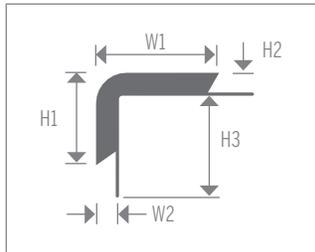
Double Butt Nosing. For butting up to carpet or tile. For use when flooring is installed on both step and riser.
