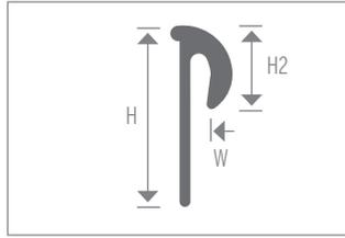
1/8" resilient cove cap for use when coving resilient floor up to 3/16" thick. Peel and stick tape for easy application.
