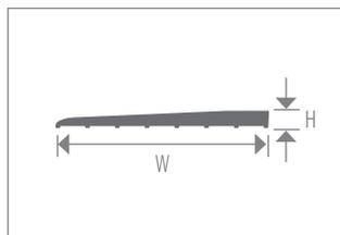
Reducer Strip for butting up to tile or resilient flooring. Provides a smooth, safe transition to substrate or adjacent flooring.
