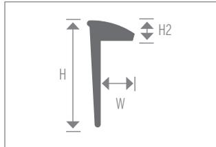
Can be used for capping carpet, ceramic, or paneling up to 1/4" thick floor.
