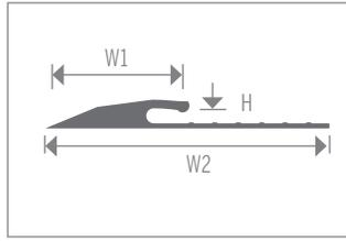
Insert Reducer for glue down carpet installations. Can be used with carpet up to 40 oz. Lip flexible up to 3/8". For heavy commercial use. Also available with 1/8" butt RD2140. Special order.
