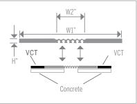
Resilient floor expansion joint cover prevents cracking in floor covering due to expansion and contraction of concrete. Ribbed section of the trim is lined up over saw cut in the slab butting up to floor covering. Use with VCT, Solid Vinyl, Rubber, Linoleum or LVT flooring.
