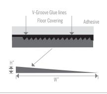
Floor Equalizer (Vinyl Reducer Strip) with V-Groove technology. Builds transition between floors up to 1/2" in height. Economical solution for height variances, quickly equalizes floor levels. Saves time and labor. Custom length sizes available. Glued, nailed and stapled directly to substrate. Floor covering can be adhered directly on top.
