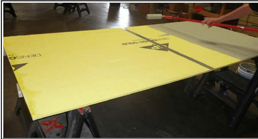
Water Resistance Test ASTM D2247
