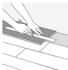
**10)** To fit the last row, lay a plank on top of the previous row. With the tongue to the wall, lay another plank upside down on the one to be measured and use it as a straight edge. Don't forget to allow room for the expansion spacers. Cut the plank and attach into position.
