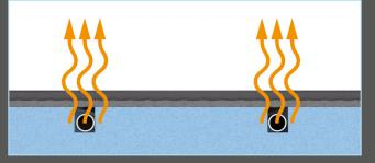
Quick heating up and cooling down Direct release of heat from the heating pipes into the tiles
