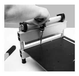
3. Attach Table Assembly (A) and Shear Assembly (B) using hardware set G.
