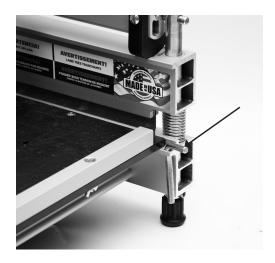
1. Press down handle and carefully remove the Cam Locking Pin. Insert Cam Locking Pin into its storage hole to prevent losing the pin. Carefully raise and release the handle.
