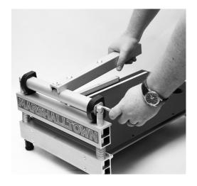
5. Attach Handle Base (C) to Shear Assembly (B) using one screw from hardware set H. Press the Handle Base (C) down and insert Cam Locking Pin (K).
