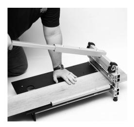
2. Place material to be cut on the table and slide past the blade to the desired length. Press flooring against the Bed Fence and hold firmly in place to ensure a clean and accurate cut. Press handle down until the blade touches the material and then firmly press down on the handle until the material is cut.
