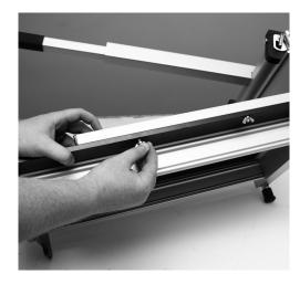
8. Place the Bed Fence (D) in two holes on the right side of Table Assembly (A) and attach using hardware set I.
