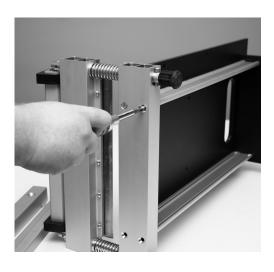
4. Attach the bed brace extrusion from the Table Assembly (A) to the Shear Assembly (B) using hardware set F.
