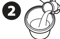
**2** Pour and scrape the ENTIRE content of **Part B** (hardener) into the mixing pail.
