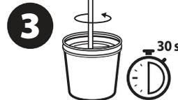
**3** Blend this A and B mixture using a low-speed mixer (approx. 300 RPM) to a homogeneous consistency (30 seconds).
