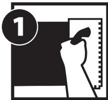
**1** Pressure-apply epoxy mortar with flat edge of notched-trowel to completely cover the substrate.
