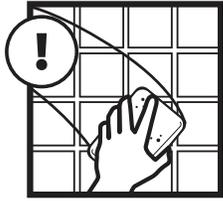
**NOTE:** Ensure that the setting material has completely cured prior to grouting. Tile surfaces and grout spaces must be thoroughly cleaned, dried and vacuumed prior to grouting. Pre-seal when required with PRO GROUT™ EASE to aid in the cleaning process and prevent potential staining.
