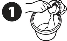
**1** Pour and scrape the ENTIRE content of **Part A** (resin) into the mixing pail.
