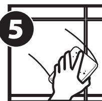
**5** Clean joints and tile face, removing smudges immediately as you go, using a damp towel before material hardens. Do not leave any residual material to remain on the tile surface as it may be extremely difficult to remove once hardened. Wash tools with water and hands with soap and water while material is still fresh.
