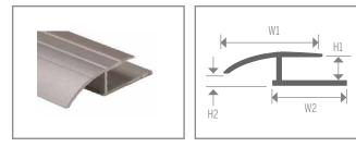
One piece floating floor Reducer. Used when butting floating floors up to 1/8" tile or resilient sheet goods. The large overhang allows the laminate floor to expand and contract up to 1/2".
