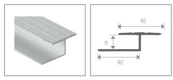
One piece Expansion Joint (divider) for floating floors. Used when installing large areas of floating floors as an expansion joint. Large overhangs allows expansion of floors and eliminates buckling. Should be used for any installation greater than 12' in any one direction.
