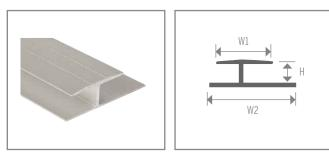
One piece Expansion Joint (divider) for floating floors. Used when installing large areas of floating floors as an expansion joint. Large overhangs allows expansion of floors and eliminates buckling. Should be used for any installation greater than 12' in any one direction.
