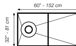
**Note:** Tray 4 features off-center drain placement: 10" (25.4 cm) o.c. from end of tray.
