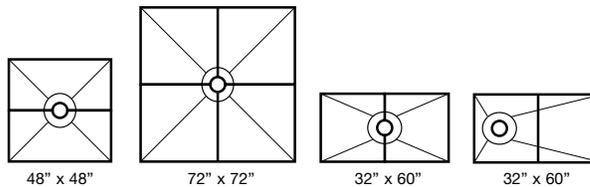
**Note:** This tray features off-center drain placement: 10" (25.4 cm) o.c. from end of tray.
