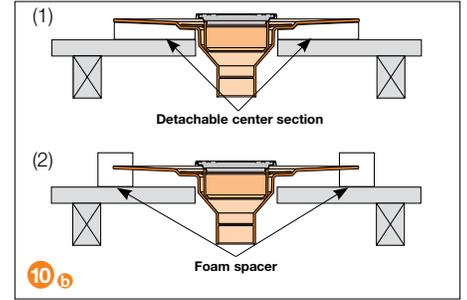
**Note:** Schluter®-Systems recommends installing the KERDI-SHOWER-ST tray prior to setting KERDI-DRAIN whenever possible. This allows greater control over the final position of the drain and makes it easier to obtain full support under the bonding flange.
