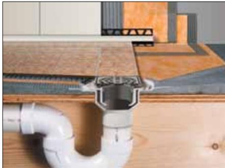
**12** The grate assembly is installed in conjunction with the tile. Place the height adjustment collar inside the lateral adjustment ring and snap the grate into place. Fill the step in the bonding flange with thin-set mortar and back-butter the underside of the grate to ensure full support. Press the assembly into the mortar and install the surrounding tiles. Position the grate to match the joint pattern of the tile covering and press flush with the tile surface.
