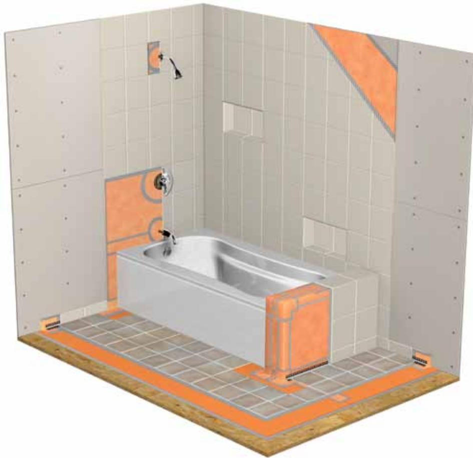
Floors can be made fully waterproof with Schluter®-DITRA. Since the membrane is made of waterproof polyethylene, the only extra step necessary is to seal the seams and floor/wall connections with KERDI-BAND. The same practice is used to integrate the DITRA with the Schluter®-KERDI used to waterproof the shower or tub surround. The result is a comprehensive waterproofing system that protects against moisture penetration.
