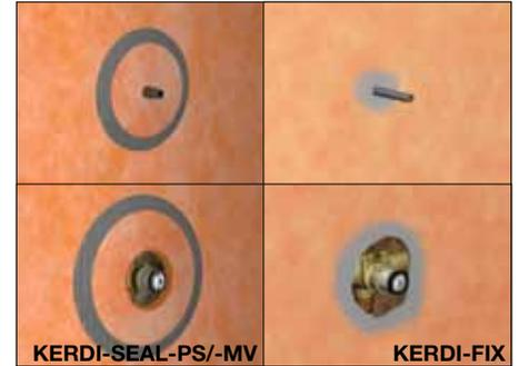
**10** Install KERDI-SEAL-PS pipe seals at shower-head, body sprays, etc. and KERDI-SEAL-MV mixing valve seal at the mixing valve. As an alternative, KERDI-FIX or equivalent sealant can be used to seal pipe protrusions and protect moisture-sensitive solid backing panels at the mixing valve.
