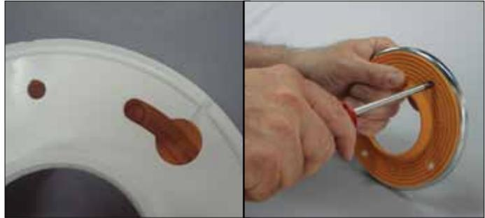
2 Align the bolt pattern of the clamping ring with the matching punch-outs in the adaptor ring. Punch the matching inserts out through the stainless steel adaptor ring.
