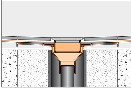
**1b** Fill in box-outs in concrete floors with dry-pack mortar. A 4" (100 mm)-diameter plastic pipe coupling or similar can be used as a form around the waste line. Select form to accommodate the KERDI-DRAIN bonding flange. Limit the hole diameter to 5" (125 mm) maximum to ensure proper support of the tile assembly.
