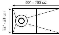
**Note:** Tray features off-center drain placement: 10" (25.4 cm) o.c. from end of tray.
