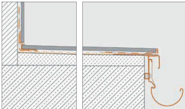
Balcony assemblies with waterproofing, integrated gutter, and waterproof wall connections can easily be built using Schluter products, as indicated.
