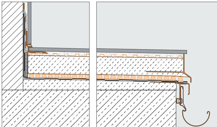
Schluter products make it easy to construct functional balcony coverings that include subsurface drainage, uncoupling/waterproofing, tightly sealed wall joints, and gutters.
