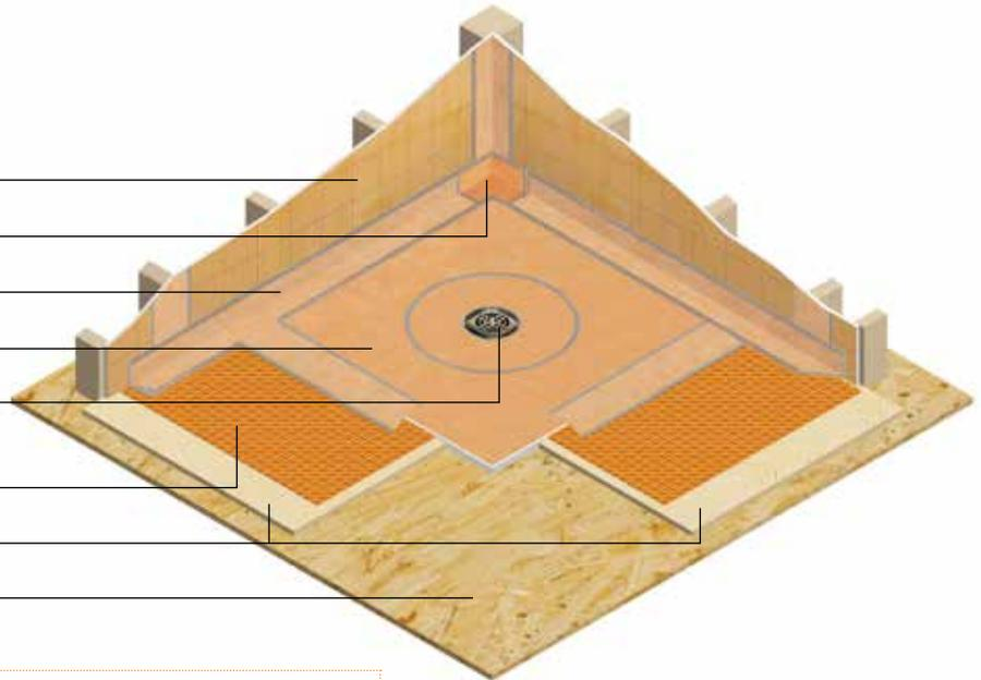
**If working with a concrete subfloor**, use a bonded mortar bed of appropriate thickness to build up the rest of the bathroom floor.
