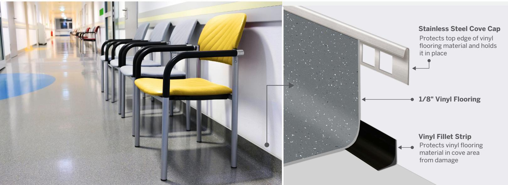
**STAINLESS STEEL COVE CAP** protects the top edge of sheet vinyl flooring material and holds it in place in a uniform manner along the wall. It is ideal for use in industrial and sanitary settings, where hygiene is a priority, and is designed to accommodate installations of flooring material up to 1/8" (3 mm). Install CM332 in combination with Fillet Strip (FL3010, FL3020 & FL3030) to protect vinyl flooring material from cracking or being punctured along floor-to-wall joints.
