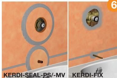
**6** Any protrusions through the KERDI membrane (e.g., mixing valve, shower head, etc.) must be sealed with KERDI-SEAL-PS/-MV, KERDI-FIX, or other suitable sealant.
