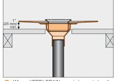
When KERDI-DRAIN must be set by the plumber prior to the mortar bed (or when there is no access to the plumbing from below), the KERDI-DRAIN is connected to the waste line and set at the desired height. When installing KERDI-DRAIN over wood substrates, the minimum thickness of mortar required at the perimeter of the bonding flange is 1" (25 mm). Before installing the mortar bed, pack loose mortar under the drain up to the inlet hole to ensure solid and uniform support of the bonding flange.
