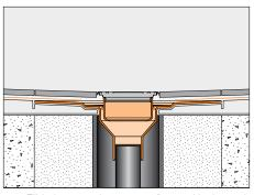
Fill in box-outs in concrete floors with dry-pack mortar. A 4" (100 mm)-diameter plastic pipe coupling or similar can be used as a form around the waste line. Select form to accommodate the KERDI-DRAIN bonding flange. Limit the hole diameter to 5" (125 mm) maximum to ensure proper support of the tile assembly.
