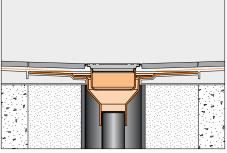
Fill in box-outs in concrete floors with dry-pack mortar. A 4" (100 mm)-diameter plastic pipe coupling or similar can be used as a form around the waste line. Select form to accom-modate the KERDI-DRAIN bonding flange. Limit the hole diameter to 5" (125 mm) maxi-mum to ensure proper support of the tile assembly.
