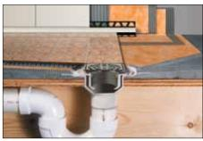
The grate assembly is installed in conjunction with the tile. Place the height adjustment collar inside the lateral adjustment ring and snap the grate into place. Fill the step in the bonding flange with thin-set mortar and back-butter the underside of the grate to ensure full support. Press the assembly into the mortar and install the surrounding tiles. Position the grate to match the joint pattern of the tile covering and press flush with the tile surface.
