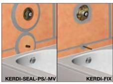
Install KERDI-SEAL-PS pipe seals at tub spout, showerhead, body sprays, etc. and KERDI-SEAL-MV mixing valve seal at the mixing valve. As an alternative, KERDI-FIX or equivalent sealant can be used to seal pipe protrusions and protect moisture-sensitive solid backing panels at the mixing valve.
