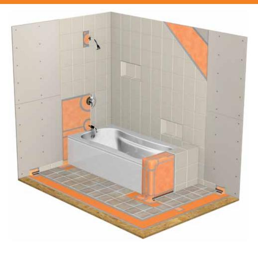
Floors can be made fully waterproof with Schluter®-DITRA. Since the membrane is made of waterproof polyethylene, the only extra step necessary is to seal the seams and floor/wall connections with KERDI-BAND. The same practice is used to integrate the DITRA with the Schluter®-KERDI used to waterproof the shower or tub surround. The result is a comprehensive waterproofing system that protects against moisture penetration.
