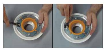
Bolts are to be finger-tight plus 1/4 turn. Do not overtighten, as this may warp the adaptor ring and result in leaks. Use star pattern when tightening bolts.
