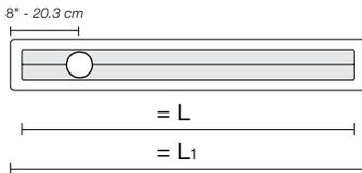
**8.7 Schluter®-KERDI-LINE** Bonding flange - stainless steel - center outlet
