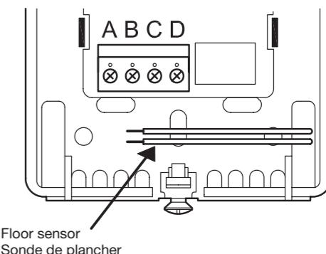
Thread the floor sensor cable through the hole in the power base.
