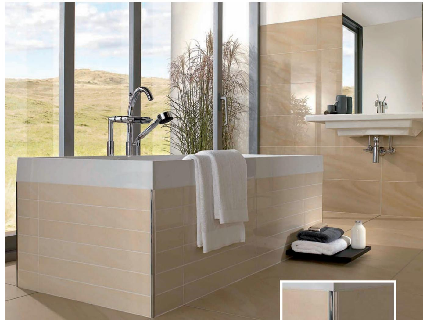
**ABOVE:** Schluter®-ECK-E edging profile in stainless steel applied to the outside corners of the bathtub skirting. **OPPOSITE:** Schluter®-SCHIENE in polished brass applied to the niche.
