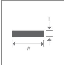
Shim - when used in conjunction with each other - can accommodate installation of the MDF moldings with floors up to 15 mm thick.
