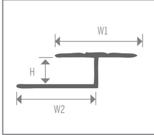
One piece Expansion Joint (divider) for floating floors. Used when installing large areas of floating floors as an expansion joint. Large overhangs allows expansion of floors and eliminates buckling. Should be used for any installation greater than 12' in any one direction.
