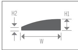
Reducer molding for reducing flooring materials such as ceramic or hardwood. Gives smooth transition from lower to higher floors.
