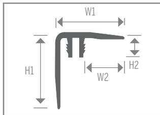
Stair Nosing finishes edge of stair. For nosing applications use LM3002, LM3003 or LM3004 track.
