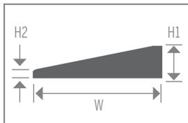
Reducer. Used when butting floating floors up to 1/8" tile or resilient sheet goods. Items supplied **undrilled**.
