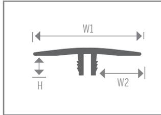
Expansion Joint (Divider) for floating floors. Used when installing large areas of floating floors as an expansion joint. Overhang allows expansion of floors and eliminates buckling. Should be used for any installation greater than 12' in any one direction.
