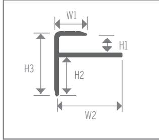
One piece floating floor Stair Nosing. Used when installing floating floors on stairs. Can also be used with ceramic tiles or other floors of similar thickness.
