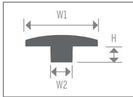
T-molding for joining adjacent floors of equal height 1-3/4" wide.
