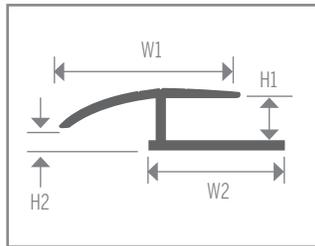
One piece floating floor Reducer. Used when butting floating floors up to 1/8" tile or resilient sheet goods. The large overhang allows the laminate floor to expand and contract up to 1/2".
