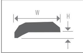
Equalizer. Joins adjacent floor height differentials. Items are supplied **pre-drilled** with a sanded but unfinished surface.
