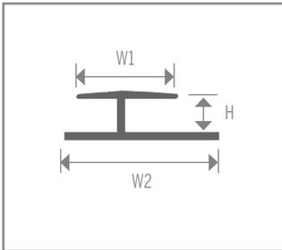
One piece Expansion Joint (divider) for floating floors. Used when installing large areas of floating floors as an expansion joint. Large overhangs allows expansion of floors and eliminates buckling. Should be used for any installation greater than 12' in any one direction.
