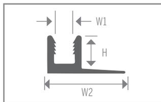
Track to be used for laminate floors. Track provides secure grip of molding for greater durability and safety. Flange adds extra strength and stability. Made of rigid PVC.
