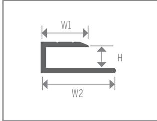
One piece floating floor End Stop (J-Mold) used when butting floating floors to walls, patio doors or other flooring materials of similar heights such as hardwood or ceramic tile.
