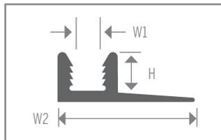
Track to be used for laminate floors. Flange adds strength and stability. Staggered drilled. Made of rigid PVC.
