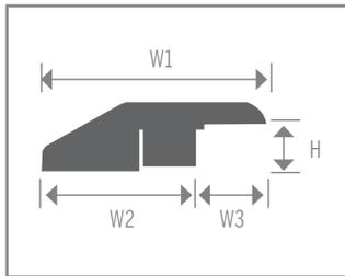
Finishes edge between laminate/wood flooring and other hard surface or carpet. Finishes edge at outside doors.
