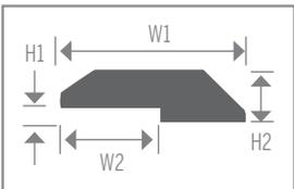
Overlap Edging. For use with resilient floors or tile up to 1/8". Items are supplied **pre-drilled** with a sanded but unfinished surface.
