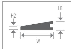
Reducer molding for reducing 3/4" flooring materials such as ceramic or hardwood. Gives smooth transition from lower to higher floors. Joins adjacent floor height differentials. Items supplied **undrilled**.
