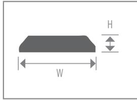
Seam binder for joining adjacent floors of equal height 1-3/4" wide.
