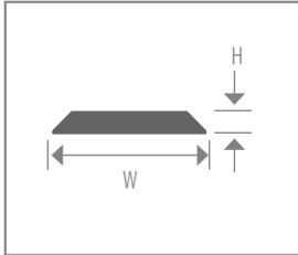
Seam binder for joining adjacent floors of equal height. Items are supplied **pre-drilled** with a sanded but unfinished surface.
