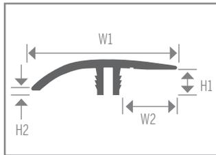
Floating Floor Reducer. Reduces from 5/16" to 1/8" floor. Used when butting floating floors on top of existing floors, subfloor, floor tile or resilient sheet goods.
