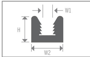
The easy to install LM3001 snap-in track design. Made of rigid PVC.
