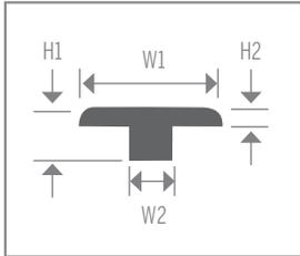
T-Molding. Joins adjacent floors of equal heights. Items supplied **undrilled**.
