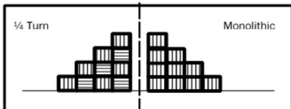
The diagram shows quarter turn and monolithic installation methods: For the monolithic method all backing arrows should point in the same direction. For the quarter turned method the backing arrows should be at a ninety degree angle to each other with all vertical arrows pointing in the same direction and all horizontal arrows pointing in the same direction at a ninety degree angle to the vertical arrows.
