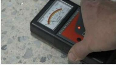
Perform a concrete moisture level test using a moisture meter or a plastic sheet.
