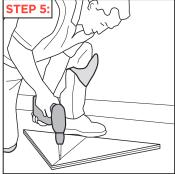
Build a Template with a plywood sheet (D). The dimension of the square template must be around 25" wide with both 90° sides. Then, place the template in the center of the room. Place the top corner of the pattern on the line B. Screw it at the subfloor to keep him in place during the installation. Make sur that you're perfectly aligned.
