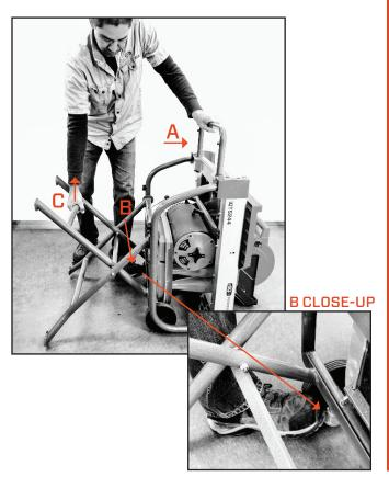
5. When X-Stand lock pin is released rotate up (A) then lift with left-hand (B) unhooking X-Stand from machine.
