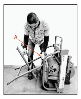
2. Put slight pressure on transport handle (A) while pushing X-Stand down (B) until lower cross bar of saw tube frame engages with X-Stand lock pin.
