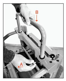
4. With X-Stand attached lifting the machine to its upright operating position. As shown below, with left foot placed near cutting head (A) with left hand lift on cutting head handle while guiding upward rotation with right hand on transport handle (C). **Note:** Before lifting allow approximately 6ft. / 2m to lift and rotate the machine to its upright operating position.
