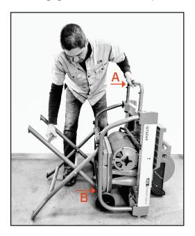
3. Lower the transport handle by pulling transport handle lock pin (A) then pushing down on transport handle (B).
