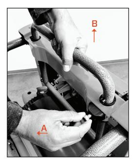
4. With slight pressure against transport handle (A) with tip of left foot pushed down on X-Stand lock pin knob (B) then pull up with right-hand (C).
