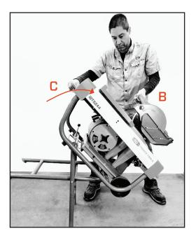
2. Guide machine back to rest softly on the floor.
