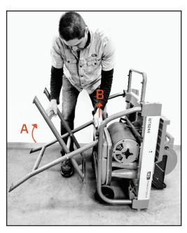
6. Machine can now be tipped forward onto the wheels for easy transport.
