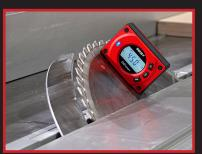
Digital measurement of gradients and angles
