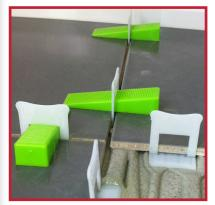
LEVTEC Tile Leveling System is designed to reduce or eliminate lippage when installing large format tile. By using LEVTEC, you can ensure the best possible result with minimal effort. Simply insert the self spacing clip below the tile then insert the wedge through the opening. Apply pressure to the wedge until adjacent tiles are flush.
