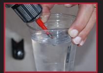
Dip in water to extend bit life
