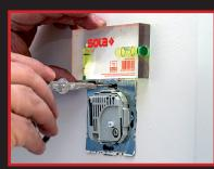
The R 100 has both a horizontal and a vertical vial and has a maximum measuring tolerance of 0.001 in./ in. (±1 mm/m, 0.057°) for precise measurements.
