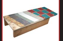
1. Clean surface from oil, water, wax and dust. 2. Spread TAVY Thin-Skin #007 Glue 3. Install TAVY Thin-Skin Underlayment 4. Skim-coat surface with any thin-set mortar (allow to dry) 5. Start setting tile
