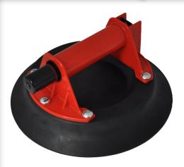
Durable handle provides easy grip. Attaches easily to a variety of surfaces. Red-line indicator warns user of any vacuum loss. Check valve allows repumping without loss of remaining vacuum.
