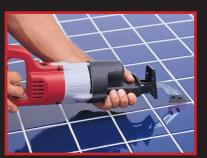
Turn a reciprocating saw into a grout removal tool
