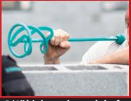
3/4" high grade steel shafts for stability and no flex
