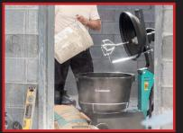
The fold down bucket cover lid is designed for safety, minimizing dust, and includes a dust extraction hook up. If opened, the paddles will stop operating.
