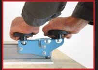
Two-handed scoring provides optimum pressure
