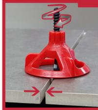
Easily spin the Leveling Cap down to the tile surface and tighten to perfectly align tiles.
