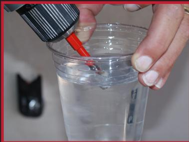
Dip in water to extend bit life
