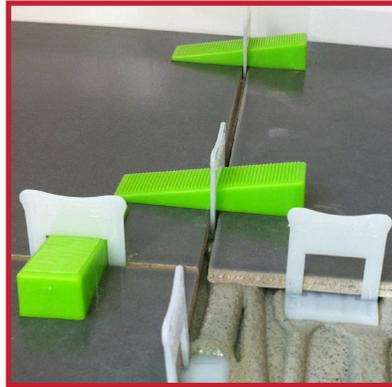
LEVTEC Tile Leveling System is designed to reduce or eliminate lippage when installing large format tile. By using LEVTEC, you can ensure the best possible result with minimal effort. Simply insert the self spacing clip below the tile then insert the wedge through the opening. Apply pressure to the wedge until adjacent tiles are flush.
