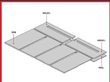
Choose small or large Filler Kit based on linear drain length
