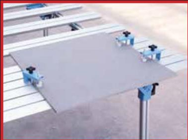
Clamp your work piece for safety during fabrication
