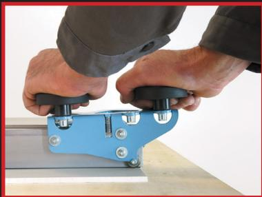
Two-handed scoring provides optimum pressure
