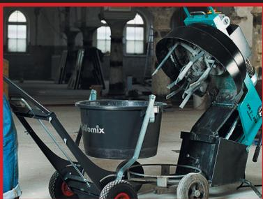
**Planetary gearing converts power into high torque and high speed, ensuring optimum mixing in the shortest time possible.**
