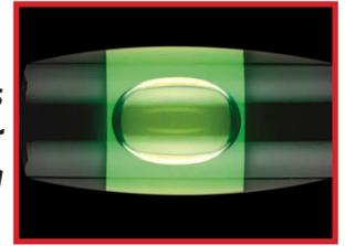
**Luminous Vial:** Every horizontal SOLA FOCUS vial is equipped with a luminous backing beneath the vial. This fluorescent light plate enables easier reading in low light situations without any LEDs. Vials are made of break-resistant acrylic material. Besides its resistance to deformation or breakage, the acrylic is highly UV resistant. Our patented ultrasonic welding of the vials ensures no leaks.
