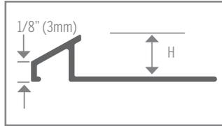
Tile Reducer has a sloped face to create a smooth transition between tile and adjacent surface such as resilient tile or sheet goods. Pre-punched for easy setting into adhesive
