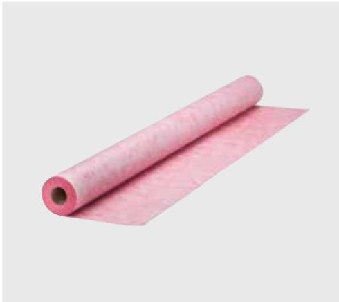
PROVA-MAT® is a thin polypropylene waterproofing membrane designed to be applied with Polymer Modified Thin Set Mortar under ceramic or stone tile to most common substrates. Unlike liquid applied waterproofing products, tile can be installed immediately onto the PROVA-MAT®. The PROVA-MAT® also provides a vapor barrier ideal for steam room and sauna applications.
