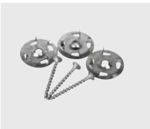
PROVA BOARD PLUS® screws and washers must be used together for a safe, simple and durable PROVA BOARD PLUS® panel installation. They are to be used to fasten PROVA BOARD PLUS® panels to wood stud framing and other substrates suitable for screw connections.
