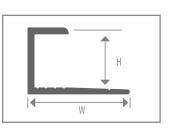
J-Molding for use with tile. Can also be used to frame glass, mirrors and wood panels.
