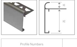
Counter top/stair nose provides a decorative finish while protecting the edge of tile or stone from chips and dents. The radius top provides a round edge for a smooth, clean appearance and meets the building code for stairs. Inside and outside corners available in both sizes. Product is available in 8' lengths and is punched to accept adhesives.
