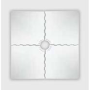
One pan solution for curbed or curbless shower installations. Pre-fabricated sloped pan with an outside thickness of 7/8" is perforated into sections for easy install and replaces the need for a mortar base.
