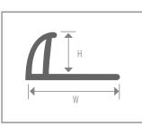
Round Heavy Duty Vinyl Tile Edge for use around bath tubs, windows, back splashes, etc. This heavy profile allows it to be used on floor tile where thinner products may not stand up to heavy traffic. Pre-punched for easy setting into mortar.
