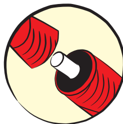
10. Ergonomic RUBIFLEX handle with 2 textures -Rigid inner core for body and consistency. -Elastic coating for better grasp and easier handling
