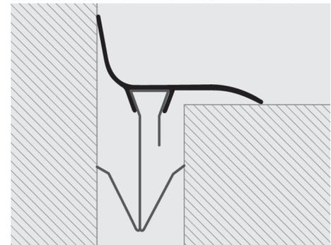
1. Choose the profile in the required width and material. 2. Insert the fixing clips into the relative groove (5 Pcs. for wall applications - 10 Pcs. for floor applications). 3. Insert/Lay the PROPLATE FIX in the existing void, applying uniform pressure or using a plastic hammer, thereby creating a perfect joint cover. The same method is used for laying the corner profile.
