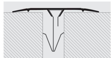
**PROPLATE FIX** is a range of flat joint-cover profiles to cover structural movements (contraction due to flexural or compressive stress) of two different load-bearing structures.
