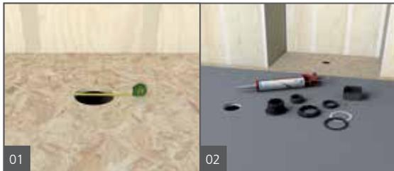
Cut the 2" (50.8 mm) pipe flush (or max. 1/8" [3.2 mm] above) to the floor construction. Make sure that the cut out fits to the Fundo panel drain. Cut out a 5" (127 mm) diameter hole around the 2" (50.8 mm) pipe to allow for the wedi drain to be inserted into the subfloor while the cut out area must remain free of deflection. The drain and trap have to be sturdily fastened to the sub floor. Assemble the drain unit following the instruction drawing.
