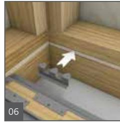
Place C brackets at the wall sides. The C brackets are installed at both ends of the recess area first, and then along the wall/side every 12 in. (center of C bracket to center of C bracket).
