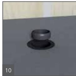
Set up the rubber caulking gasket (with the beveled side up) around the 2" (50.8 mm) pipe in the subfloor. The rubber gasket must be flush with the upper end of the 2" (50.8 mm) ABS or PVC pipe. **Do not use any lubricants.**
