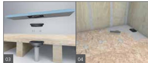
Cut the 2" (50.8 mm) pipe 1 1/4" (31.8 mm) below the top of the Subfloor. Use the oval shape cutting template where you want to position the drain to cut out subfloor using a jigsaw to allow wedi drain trap to be inserted and connected to floor pipe using appropriate ABS compatible or multipurpose cement glue. Please also check cement glue compatibility to floor pipe material. The drain and trap have to be secured to the subfloor. Drain recess cut out must not add deflection to subfloor.
