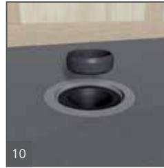
Set up the rubber caulking gasket (with the beveled side up) around the 2" (50.8 mm) pipe in the subfloor. The rubber gasket must be flush with the upper end of the 2" (50.8 mm) ABS or PVC pipe.
