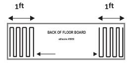
Apply FuzBond Wood "Glue Assist" 5650 (ft on both ends) as shown in diagram. Available in (20.03oz sausage tube)
