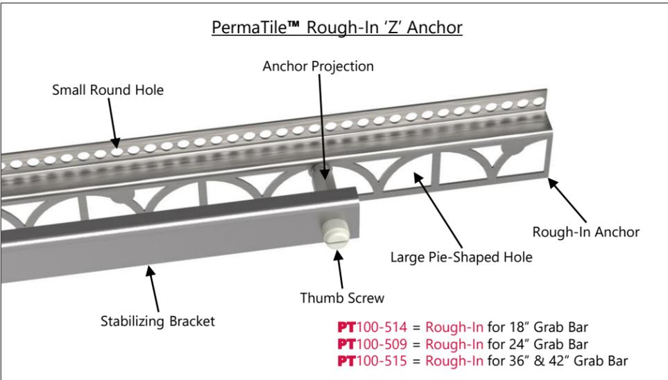
Each PermaTile™ Rough-In 'Z' Anchor is equipped with a stabilizing bracket. The bracket is a tool that guarantees that each grab bar will mount properly. The stabilizer is fixed to anchor projections with thumb screws.
