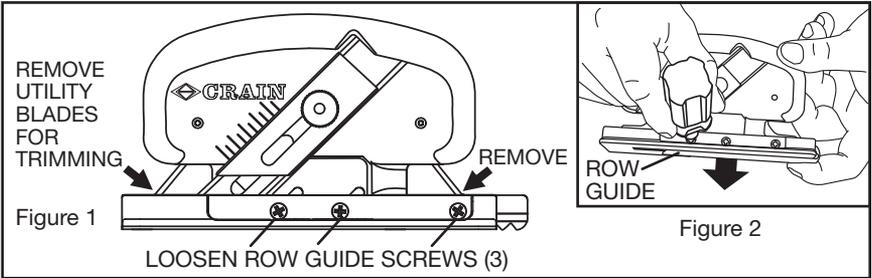
Part the nap of the carpet with a row finder or separator. Set the base of the cutter on the carpet with the extended row guide (Figure 3) inserted into the parted row (Figure 4). With some downward pressure on the handle of the tool, press the row guide down (Figure 3) to the bottom of the row. Once the row guide depth is set, retighten the 3 screws.
