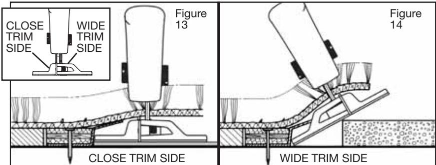
When trimming, keep the inside edge of the cutter's base pressed tight against the Z-bar. This will give you the perfect amount of carpet to fold underneath the Z-bar once the trimming operation is complete.
