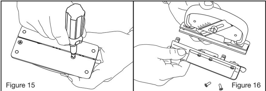
Loosen the two thumbscrews, which loosens the blade clamps. Install two utility blades as shown in Figure 17.
