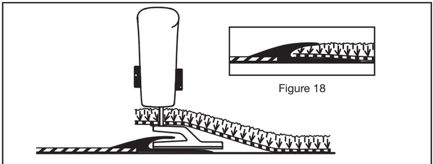
**INSTALLATION TIPS:** Glue carpet within two feet of the molding.
