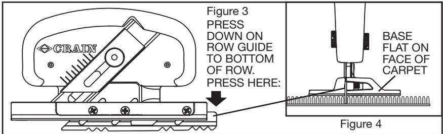
**NOTE:** The row guide should ride on the bottom of the row when the base is flat on the face of the carpet (Figure 4). The base should not teeter back and forth on the row guide. If it does, shorten the depth of the guide until there is no rocking, yet the guide still contacts the bottom of the row.
