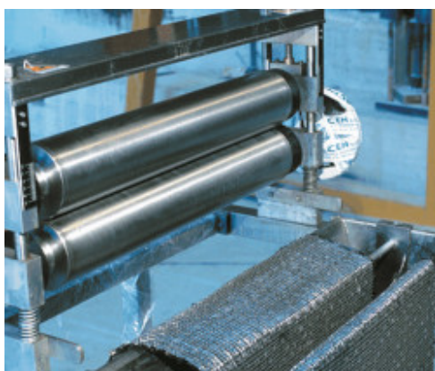
Impregnating MapeWrap C with a machine
