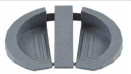
• 3 in 1 tile shim: 2 spiral-shaped wedges (lateral ones) + 1 wedge (middle one). • For joint adjustments from 2 to 10 mm.
