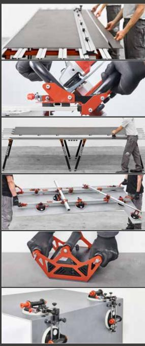
The widest and most innovative range of equipment ideal for ceramic tiles slabs. Thanks to cutting rail RAIZOR and T-CUT device it is possible to perform perfect cuts with scoring method. POWER RAIZOR and BC45 cutting units allow to perform 45° cuts (Jolly), 90° cuts and with variable angles (also 180°).
