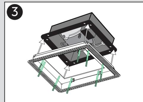
Mount fan to top of **Flush Exhaust Mount** and secure with **screws**.
