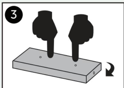
3 Hold in place. Flip tray upside down. Apply even pressure until flooring material lies flat with rim of tray.
