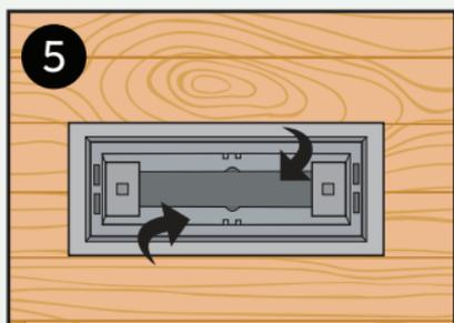
5 To open air flow, push down the dampers in body. This can be done anytime after install.
