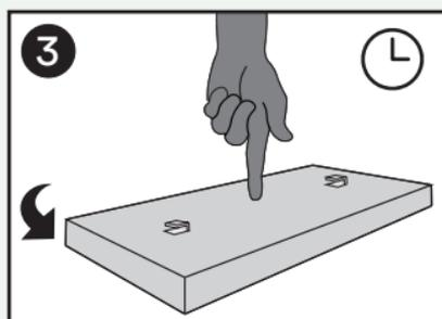
3 Flip tray and allow bonding material to cure. Ensure flooring material is flush with the rim.
