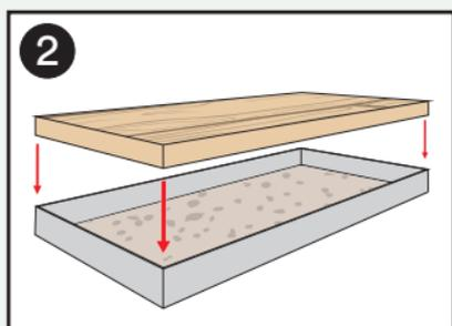
2 Apply adhesive bonding material in tray. Insert pre-cut flooring material.
