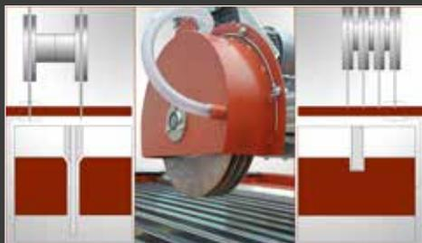
**SCIE DE PRÉCISION POUR COUPE ET BISEAU AVEC AVANCEMENT AUTOMATIQUE (DISQUE SIMPLE ET MULTI-DISQUE) MACHINES POUR APPLICATIONS SPÉCIALES**
